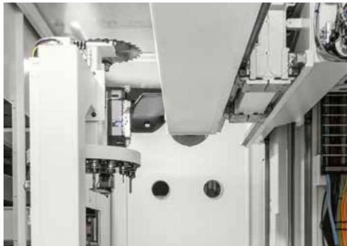
Quick tool change thanks to a motorized tool store located near the work area.
