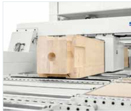
Firm and precise movement of the element by means of large self-centering clamps.
