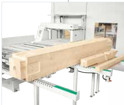
Automatic unloading of the finished element by means of a rear mechanical pusher.
