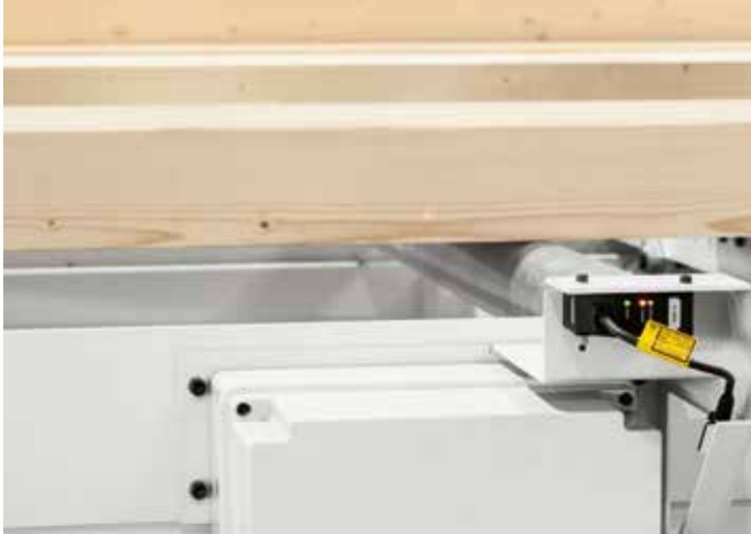
Curvature verification kit to help the machine operator.
