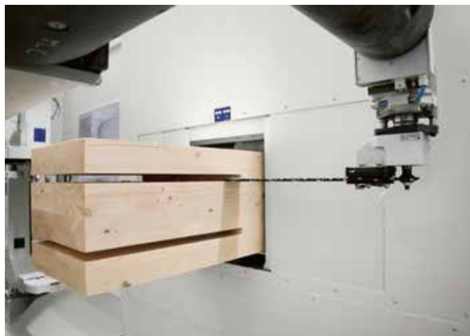
Mortise chain aggregate available for executing precise internal corner cleaning and long notches.
