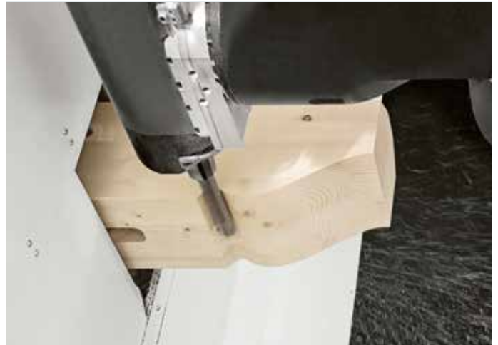
6-axis machining head unit with automatic tool change. Power: 13 kW / 25 kW (S1).
