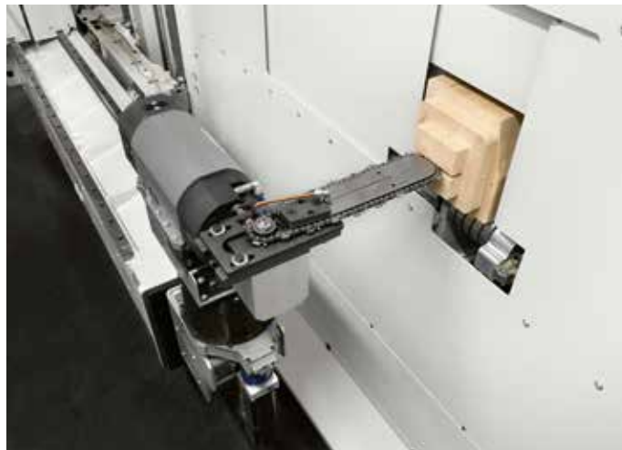
5-axis unit Flex-5 with automatic tool changer, marker and laser probe. Power 12.8 kW (S1).
