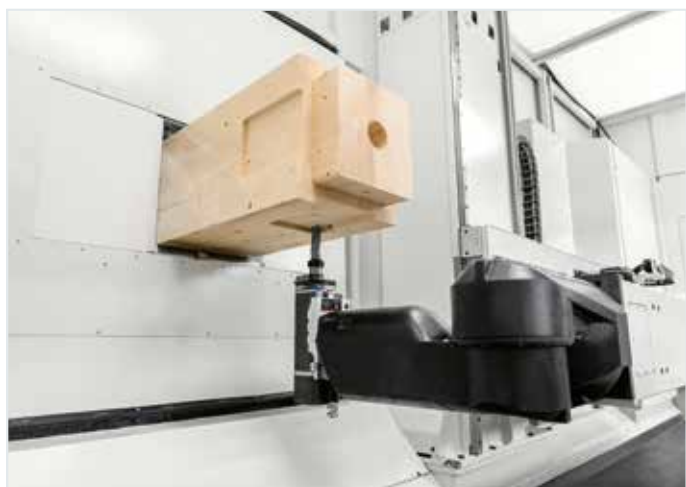
Each tool can operate on all sides of the element, ensuring complete processing.
