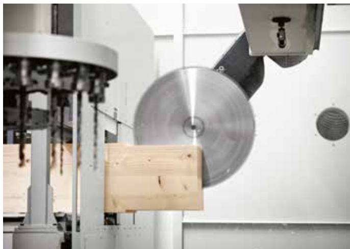
Sawblade of 740 mm diameter, perfect for executing precise cuts and deep notches for hardware fittings.
