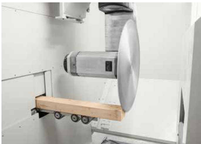
Independent sawblade unit with 240 mm cutting capacity, power 10.6 kW (S1). Dynamic workpiece support device.
