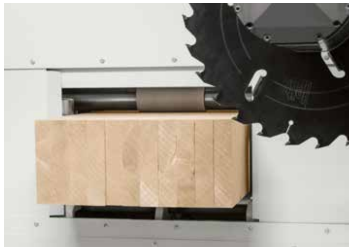
Straight beam and panel processing mode: it operates just like the Oikos X.
