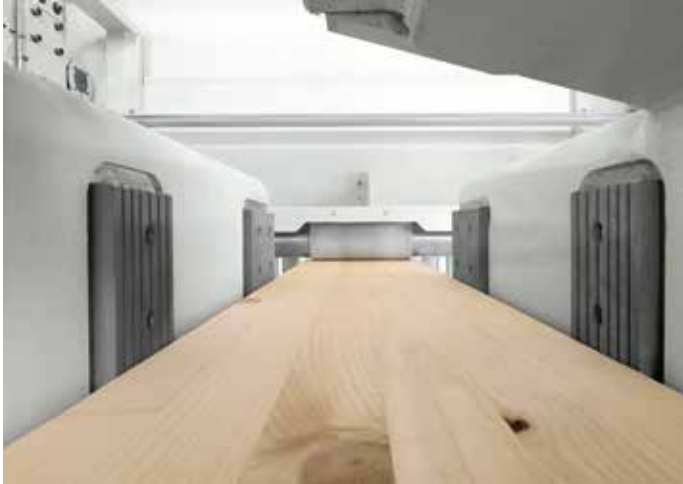
Self-centering feeding clamps that guarantee a perfect grip of the workpiece.
