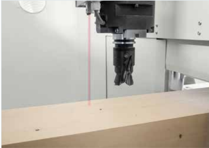
Integrated laser probe on the machining head unit ensures ultra-precise routing and drilling operations.
