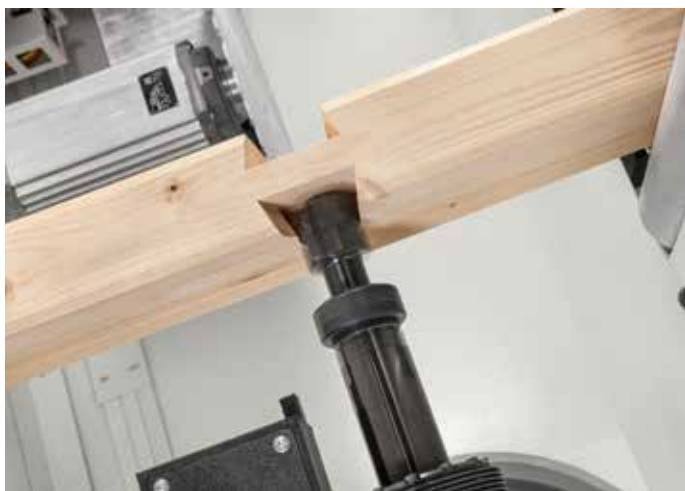
Automatic laser probing cycle, dedicated to the machining of pockets, holes and dovetail joints.
