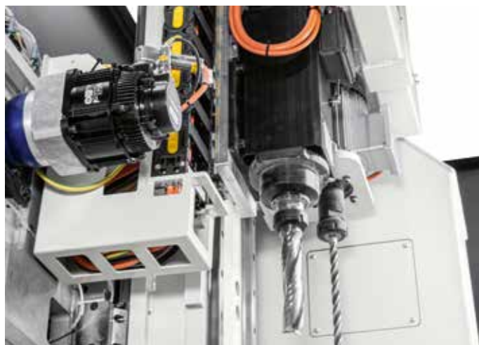
Vertical drilling and routing units with 3 axes independent movements.
