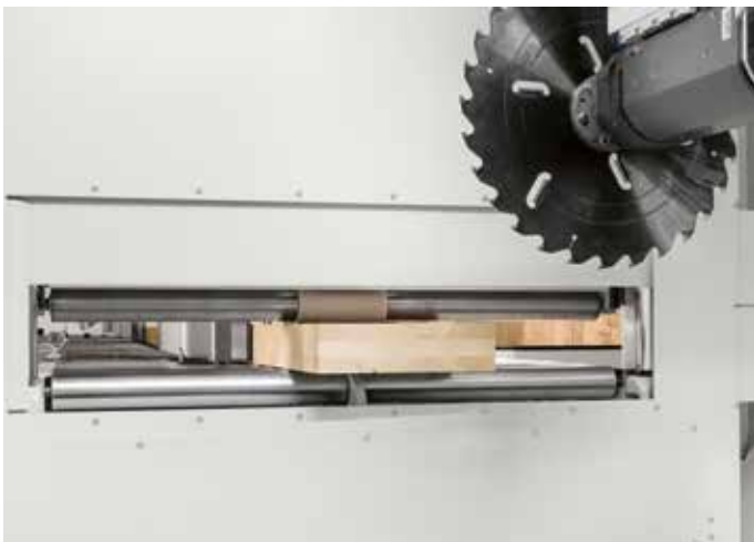
Camber beam processing mode: intelligent handling through full-stroke clamps and pressure rollers.
