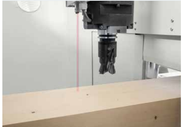
Integrated in the machining head unit laser probe , for high precision drilling and routing operations.
