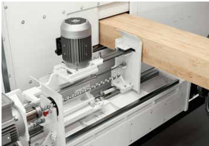
Horizontal mortising and drilling units with guide-system.
