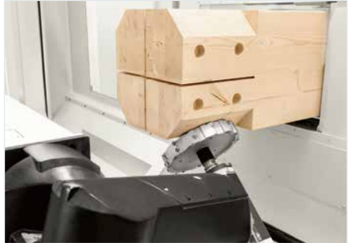
25 kW (S1) electrospindle for high-performance chip removal.
