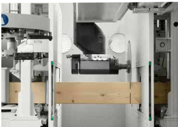
Workpiece overhang dynamically reduced thanks to symmetrical guide carriages.
