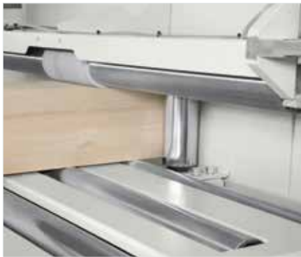
No vibrations thanks to the use of pressure rollers that secure the element during processing.
