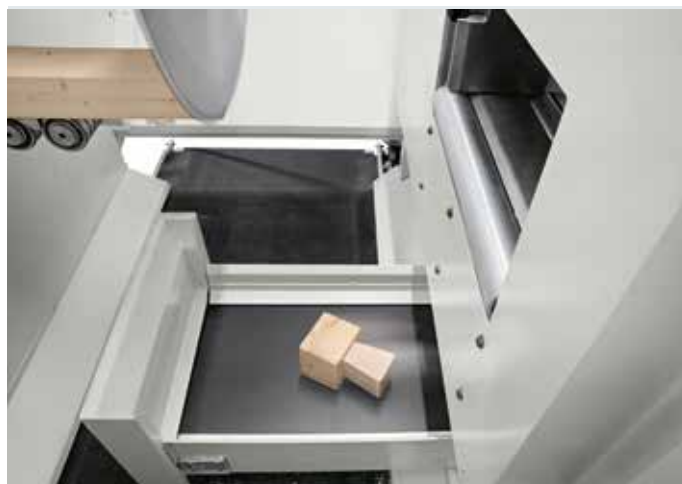
Recovery of short pieces with return to the operator, without requiring machine stoppage.
