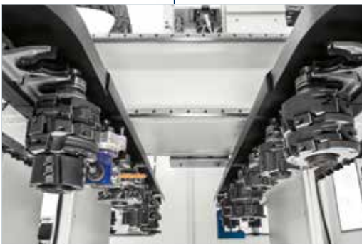
N.4 chain tool stores Superior efficiency.
