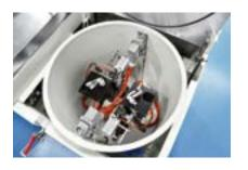
The exclusive SCM system allows the simultaneous preheating of 2 glue pots with PUR glue, directly inside the tank. In this way the glue pots are immediately ready for use.
