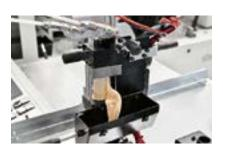
The external mounting station can accommodate a single glue pot, both motorized and powered, it allows for easy management of all cleaning, maintenance, unloading, as well as glue change operations.
