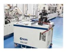
Easy cart is suitable for all glue pots available in the range, SGP-E, SGP, HGP. Completely independent from the edge bander, it can be installed in any position and easily moved where necessary. It only requires compressed air and power supply, without the use of inert gas (nitrogen) or other chemical products.
