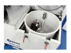
The innovative system of air management inside the tank, by means of the control software, allows the correct maintenance of the PUR glue, up to a period of at least 72\* hours.
