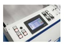
Thanks to the large "Touch Panel" control screen, all the operating modes of the new easy cart can be managed and monitored on a single screen. The independent electronic thermoregulation of up to 3 glue pots allows the change of processing in just a few minutes.
