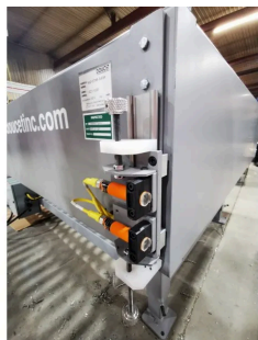
5" STROKE OPTION ON RECEPTION CONVEYOR WORKING HEIGHT WITH AUTOMATIC RECEPTION HEIGHT ADJUSTMENT
