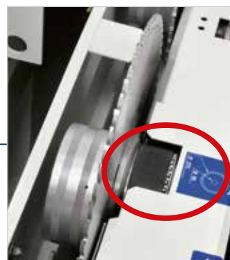
Toothed belt Transmits maximum power with low levels of vibration and abrasion.
