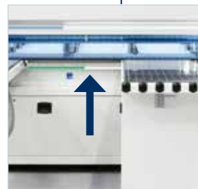
Movable air floating tables a led bar Assisted management of the positioning of the movable air floating tables according to the panel format.
