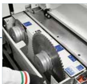
New blade carriage for easy inspection and maintenance. With maximum power up to 18 kW .
